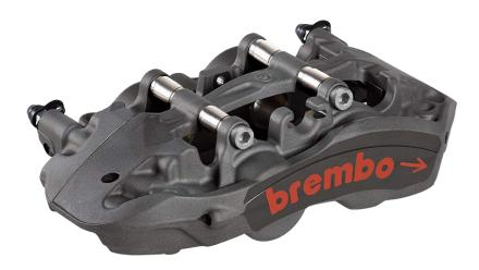
6 pistons, 28/32/38 mm (1.10/1.25/1.49"), suitable for disc diameter 356 – 380mm (14.01"– 14.96") and disc thickness 32 – 36mm (1.26" – 1.42")
