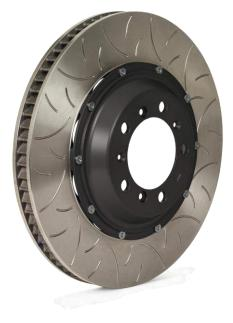
The T3 discs are characterized by an aggressive grooves machining that offers high initial response with a smooth pedal feel. The T3 discs are the most used rotors in the professional racing level and offer high bite and good modulation.
